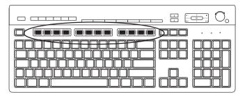
The function keys, located above the main keys, are labeled F1 through F12.
